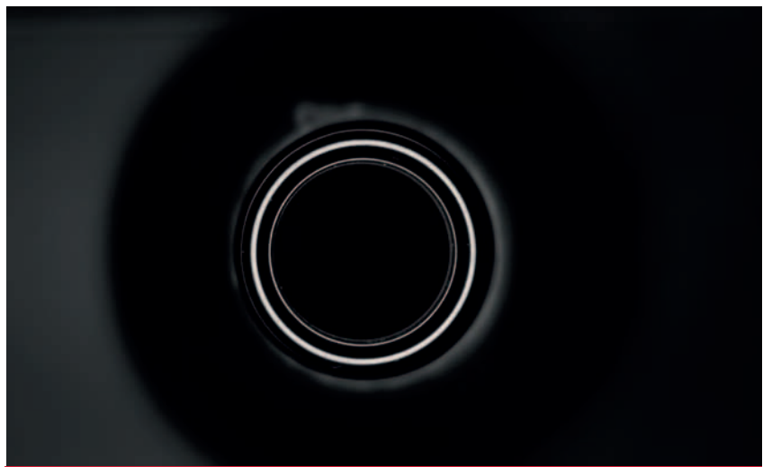
In this image of the sealing surface, the illumination is coming from the sides
